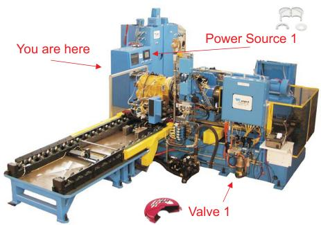
PPE Required: Light Eye Protection, Ear Defenders, Boots, Overalls Equipment Required: Circuit breaker lockout, non-conductive padlock, lockout tags
